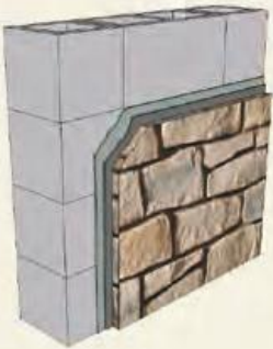
Clean Masonry Installation Scratch coat Setting bed Dutch Quality Stone™
