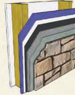
Rigid Board Installation Rigid board Weather resistant barrier Weather resistant barrier Metal lath Scratch coat Setting bed Dutch Quality Stone™
