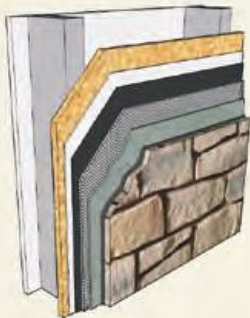
Metal Stud Installation Sheathing Weather resistant barrier Weather resistant barrier Metal lath Scratch coat Setting bed Dutch Quality Stone™
